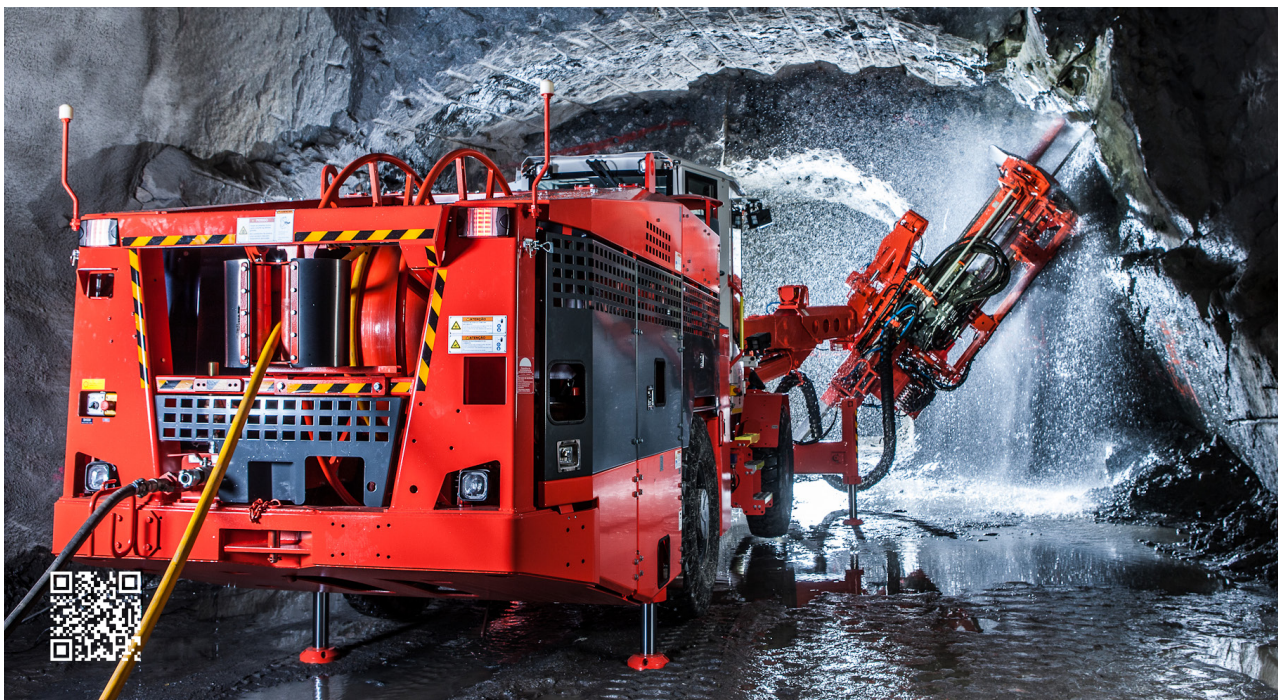
1. DL431 TOP HAMMER - LONGHOLE DRILL
